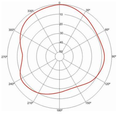
Horizontal Polar Diagram Frequency: 1 KHz
